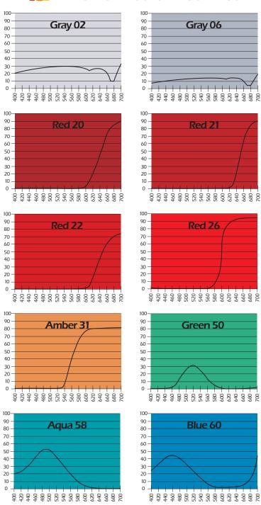
TSP color filters are available in a wide range of standard colors in both acrylic and polycarbonate. These filters are designed for use with the most commonly used displays (LCD, LED, EL, VF, etc.). TSP can also prepare filters colormatched to specific application requirements or to duplicate the color of existing filters. Choosing the proper color will provide sharp, high resolution characters with enhanced contrast between the displayed information and the background.
